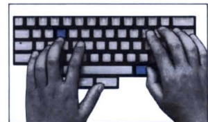
“CAPS” is on the front of [e]. To use this command you highlight the text you want to affect, hold down [USE FRONT], and, while holding it, press and release [CAPS] as shown above.
